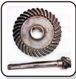
AGW 211573 CROWN WHEEL PINION 34/7 TEETH
