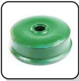
AGW 212001 BRAKE DRUM 3393285, 03393285 ID : 250MM, TEETH : 23 6006,6806,7006,7206,6807 7007,7207,7807
