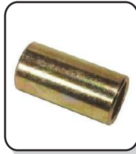
AGW 752530 LOWER LINK CONVERSION BUSH CAT 1/2 (LENGTH: 44.5MM) 81819374,C7NNG992A
