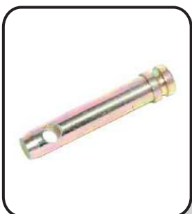
AGW 752517 TOPLINK PIN CAT2 25 X 97MM 81816506,C5NN560A C5NNF847A,E1ADDN560 E27N995248 FORD 3000,3600,3610,4000 4600,4610,5000,6600,6610 7000,7600,7610
